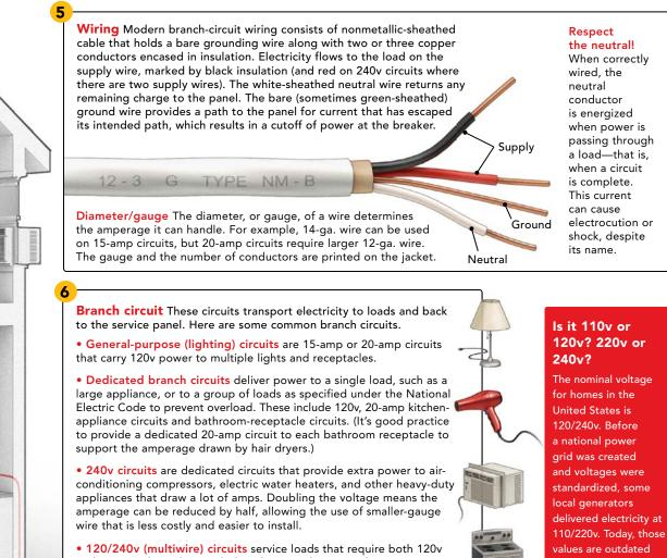
and 240v, such as electric clothes dryers and ranges. The 120v runs lights, motors, and controls, while the 240v supplies the heating elements. Amperage is typically 30 amps to 50 amps.
