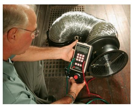
A duct blaster is not quackery. Similar to a blower door, a duct blaster is a calibrated fan. It is used on buildings with forced-air heat or central air-conditioning. Leaking ducts can decrease the overall efficiency of your heating and cooling system by as much as 20%.
